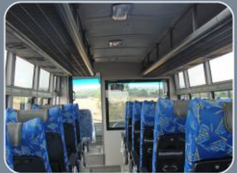
ABS interior paneling with full driver partition
